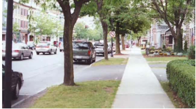
Figure 7. Sidewalks shall extend across driveways helps to create a nicer and safer pedestrian environment.
